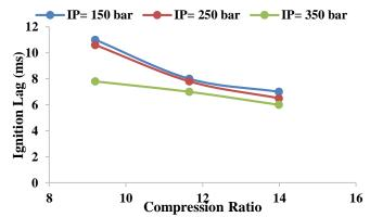
Figure 2: Variation of Ignition Delay with Compression Ratio at Different Injection Pressure for Gasoline
